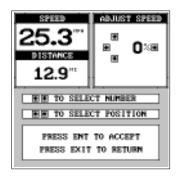
to make it read slower. Use the arrow keys to change the speed, then press the ENT key. Press the EXIT key to erase this menu.
